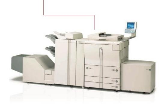
The Canon iR9070 brings unparalleled productivity and ease to on-demand, black-and-white document production. Continuous high speed output, at a fast 90 ppm, is combined with consistently excellent image quality.
